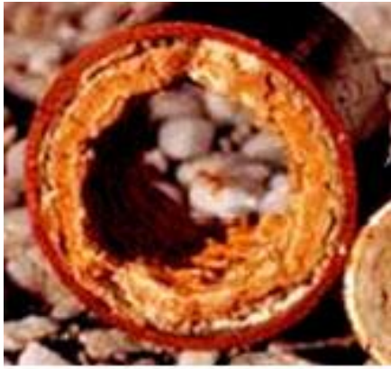
Scale buildup in a pipe, caused by hard water. Credit: Dept. of Energy.
